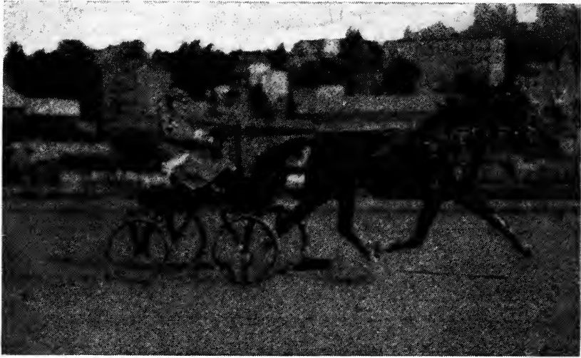
Showing the worst distortions (wheels) that will happen with a good shutter. Nettel camera. 7" F. 4.5 Tessar. 1/560 second exposure. Trotter going full speed, distance about 6 yards.
